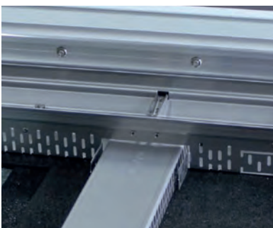
Insertion of the branch channel into the channel. It is recommended using min. 2 branch channels with a length of 50 cm per metre of channel
