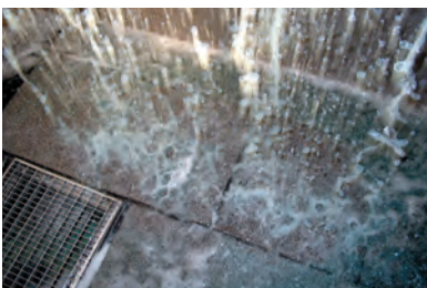
Maximum rainfall of the surface clearly shows the important function of the gully tops for roof gullies
