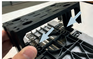
Position the springs and press the adjustment unit into the corresponding retainers.
