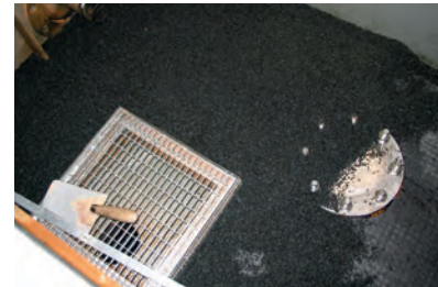
Test set-up with drainage mat and gravel bed in front of the gully top
